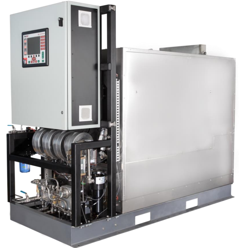
M-Series (mobility) Up to 9.8 kg H 2 /hr demonstrated. Plan to scale-up at least 2x
